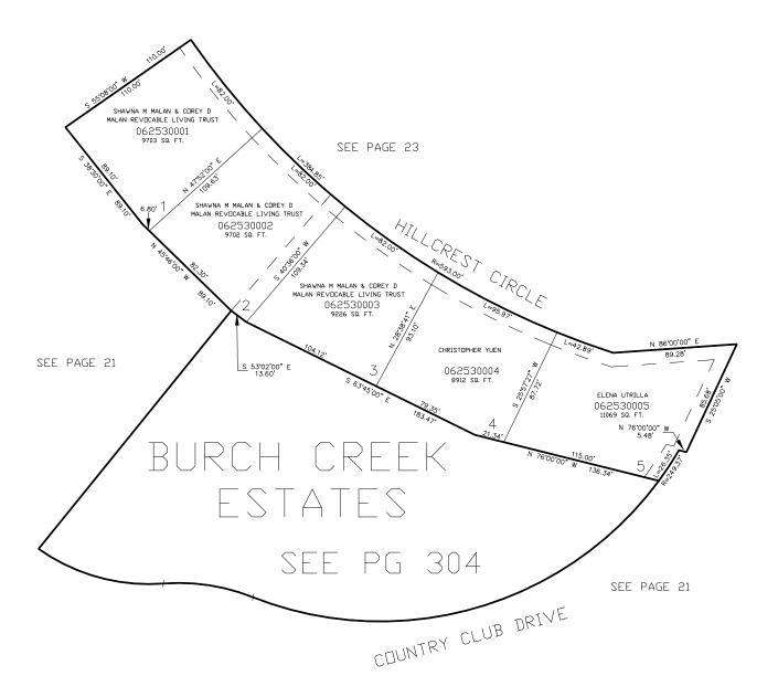
10' UTILITY & DRAINAGE EASEMENTS EACH SIDE OF PROPERTY LINES AS INDICATED BY DASHED LINES EXCEPT AS OTHERWISE SHOWN.
